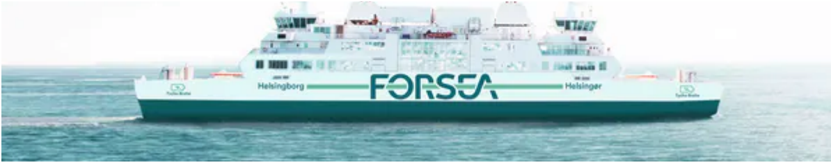
Tycho Brahe - an electric vehicle and passenger ferry with 4,000 kWh of batteries. Forsea
